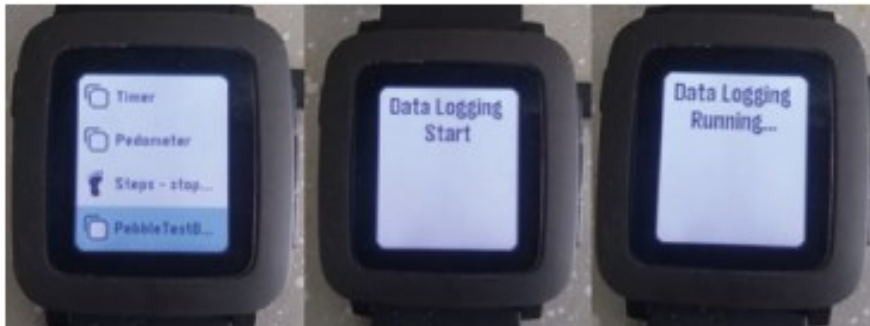
Figure 14: Pebble Time custom accelerometric acquisition app. On the left, A: OS menu selection; Center, B: App frontend before acquisition start; on the right, C: acquisition running.
