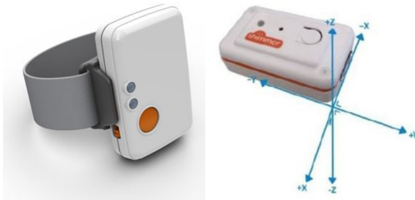
Figure 15: On the top: ShimmerSensing bracelet with technical characteristic; bottom: reference frame for the sensors.
