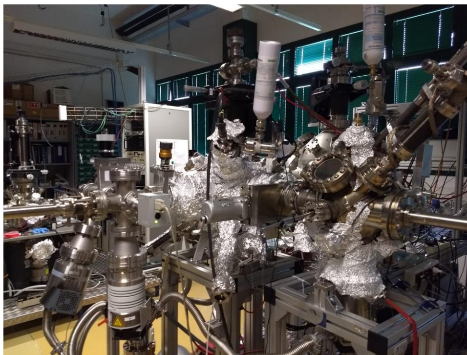
Figure 10: view of the OSMOS laboratory. On the right is the STM chamber, separated with a gate valve from the preparation chamber, where also the LEED is present.
