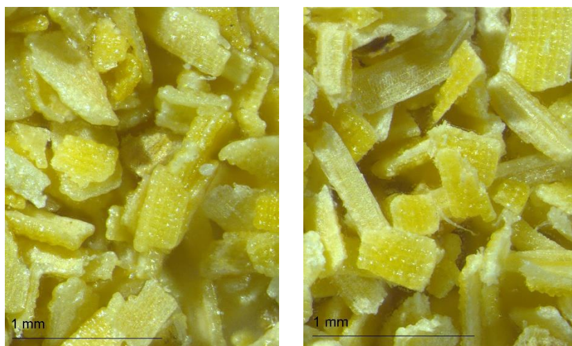
Figure S7 Comparison of the microscope images (60x) of the F-TLL-PVP immobilized lipase before (left) and after (right) 10 reaction cycles of tributyrin hydrolysis.
