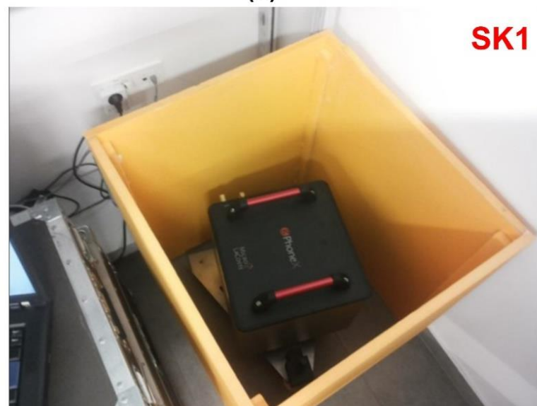
Figure 2.18 a) Location of the gravity station SK1. Blue line: Reka River path; white lines: outline of the Škocjan cave. Orthophoto from Google Earth. b) The gPhone gravimeter.
