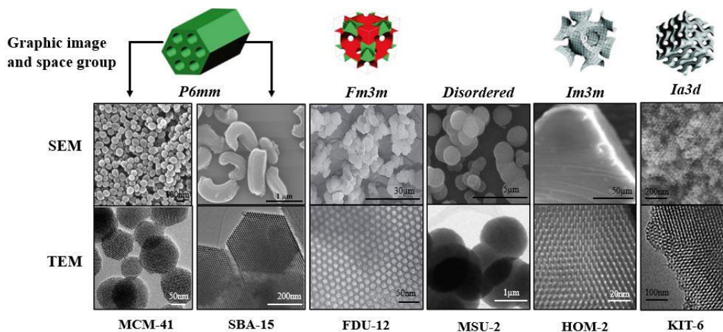
Fig. 24 SEM and TEM images of different mesoporous silica materials [100], [107], [109]–[113].
