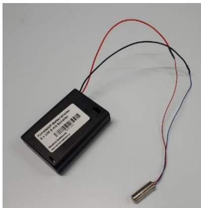
Figure 25. Photograph of commercial vibrating motor and the battery power supply installed on the peristaltic pump inlet. 56
