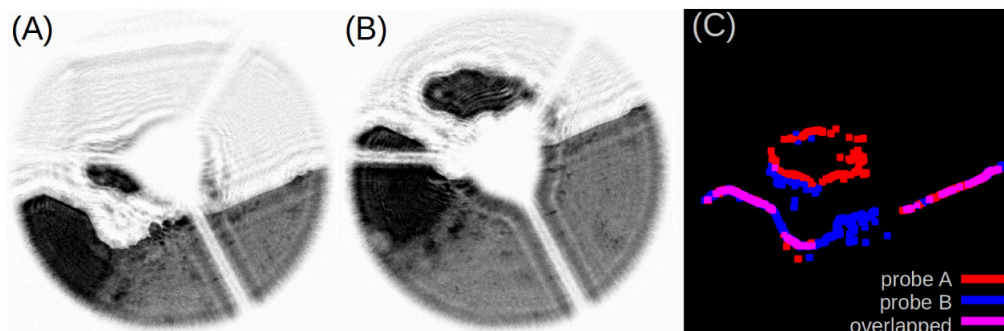
Figure 3.4: (A and B) Two neighbouring reconstructed probes for which it is necessary to know their relative position. Note in the center the presence of the beamstop and its support. The alignment/registration needs to be performed only on their common parts. Panel (C) highlights the edges from the two probes when aligned
