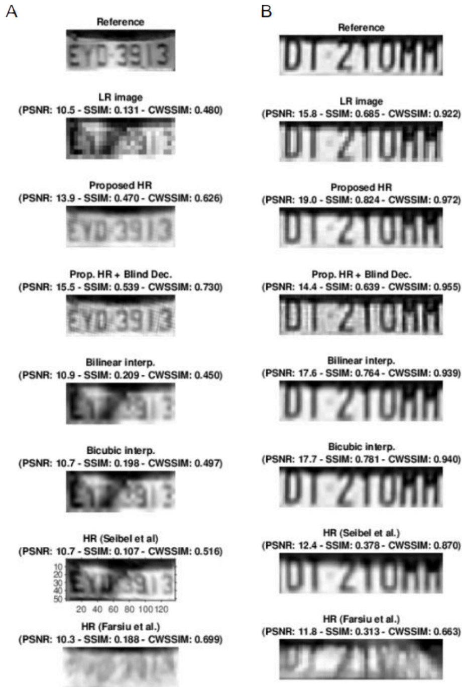
Figure 5.21: Results comparison for two samples (A) and (B). The super-resolution reconstruction (proposed method and proposed method + blind deconv) are confronted with two upsampling methods as well with other two super-resolution algorithms. The proposed method provides more contrast and allows deciphering correctly the licence plate characters.
