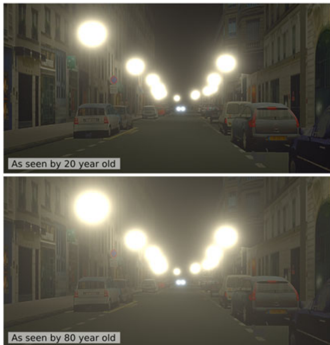
FIGURE 11 — Visualization of night vision for 20- and 80-year-old observers. Note the increased amount of glare and reduced sensitivity for the 80-year-old observer.
