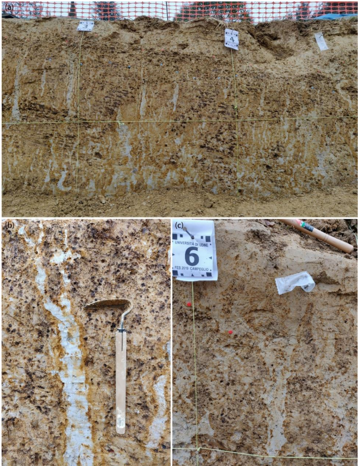
Fig. 5.10 – Details of the vertical blue-grey dikes characterizing the excavated wall. (a) Abrupt interruption of the lateral continuity of the coarse levels; (b) detail showing the yellow-reddish sandy borders and the blue-grey infill; (c) detail showing the shallow-up color gradation of the dikes, not accompanied by size gradation.
