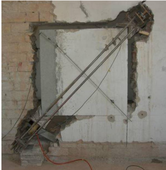
Fig. 22. Diagonal compression test.
