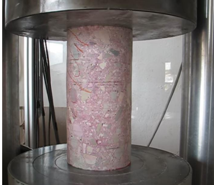
Fig. 19. Compressive strength test on cylindrical specimen.
