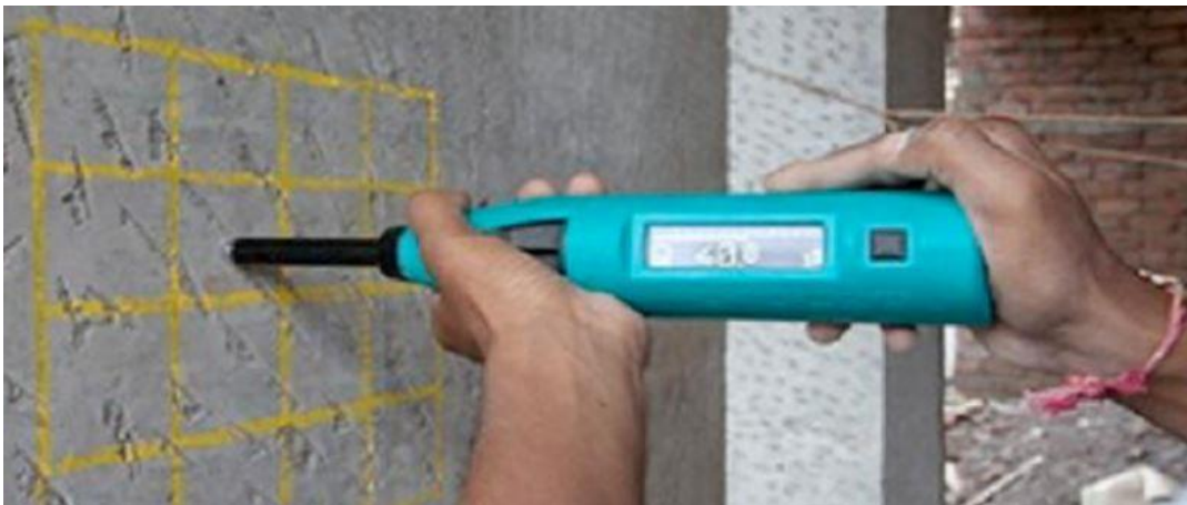
Fig. 12. Rebound hammer test.
