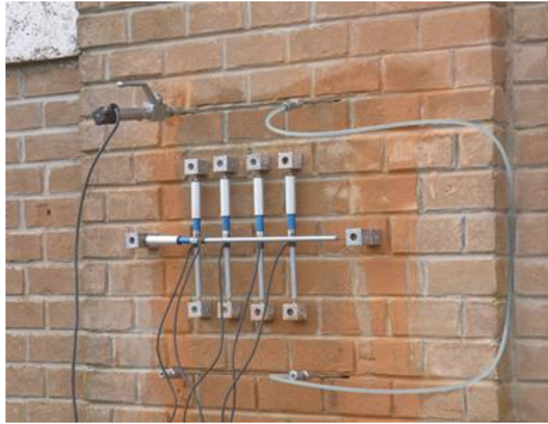
Fig. 21. Double flat jack test on masonry.
