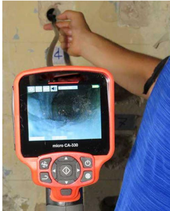
Fig. 5. Endoscopy for the evaluation of the stratigraphy.
