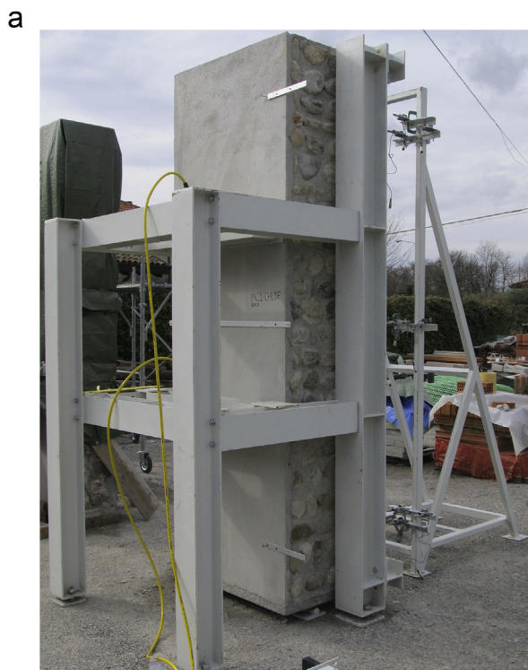
Fig. 4. Compression tests on masonry specimens: (a) test apparatus and (b) compressive stress \sigma_c vs. strain \epsilon_c curves.
