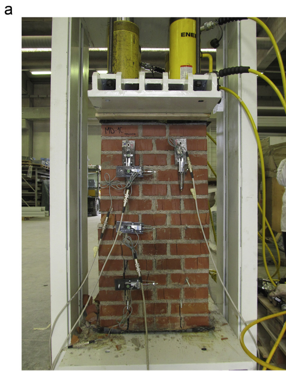
Fig. 4. Compression tests on masonry specimens: (a) test apparatus and (b) compressive stress \sigma_c vs. strain \epsilon_c curves.
