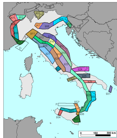
Figure 2-2: Seismogenic zonation ZS9. The blue borders separate zones with the same kinematic significate, that differ mainly for seismicity characteristics. The seismic zones (ZS) with dashed border, identified by a letter, have not been used in the hazard evaluation [17].
