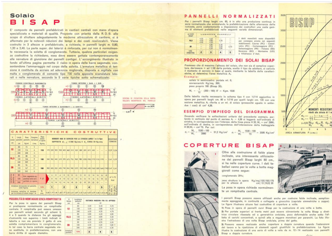
Figure 3-8: Manual of the hollow pot slab Bisap, used in most of the storeys of the case study building.
