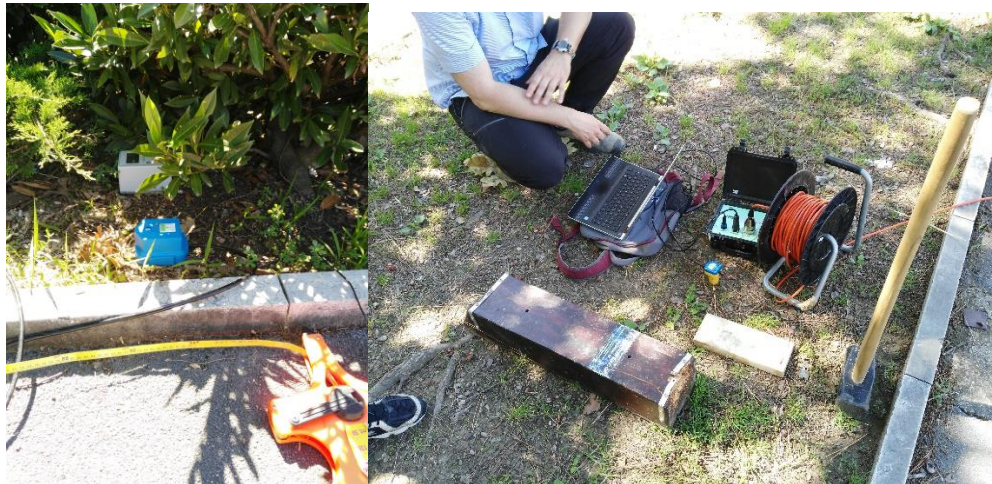
Figure 1-16: Photos from the test-site. On the left: a Tromino is visible, the meter for determining the distances between the vibration source and the instrument and a geophone that measures the same vibration. On the right: vibration source (a piece of wood and a hammer) and measuring instruments.
