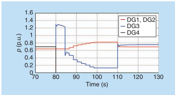
**Figure 21.** The simulated generator's active power transients during an emergency reconfiguration procedure.
