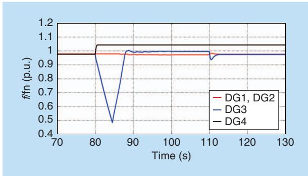
**Figure 20.** The simulated generator's frequency transients during an emergency reconfiguration procedure.
