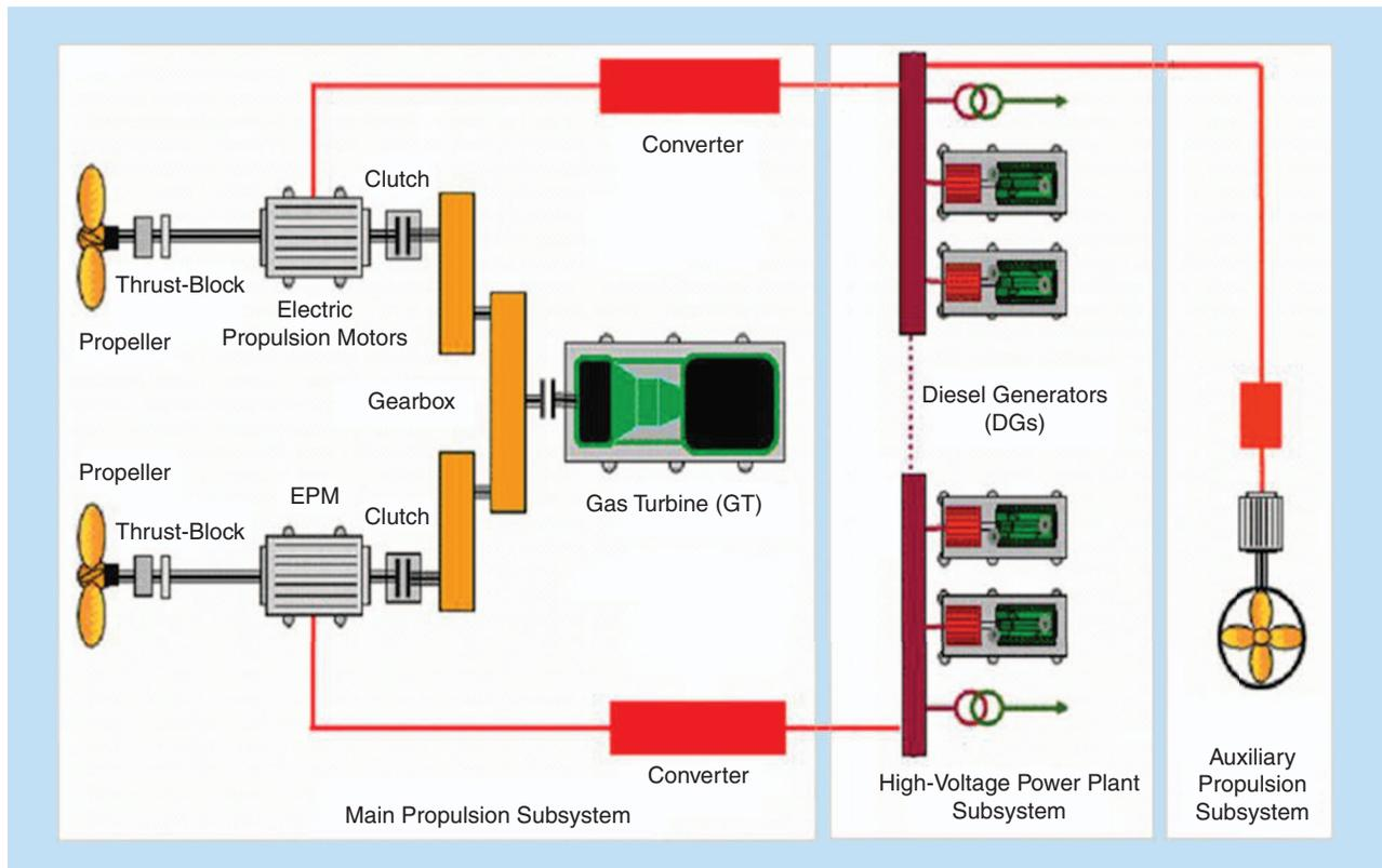
Figure 7. The ship hybrid propulsion system layout.
