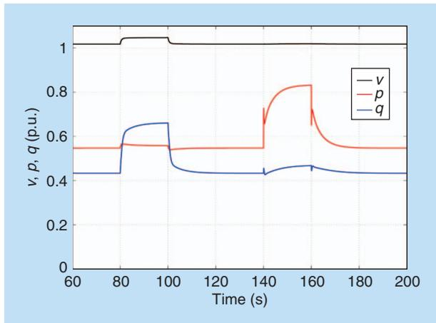
**Figure 8.** The inverter-based generator responses due to voltage and active power references step variations ( $\pm 2\%$ ).
