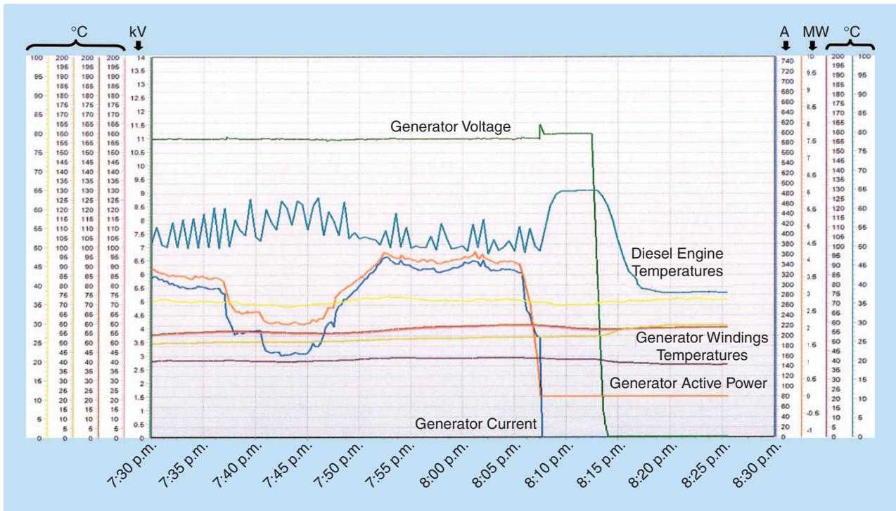
**Figure 13.** The ship's automation print screen of a generator's main variables during its disconnection.
