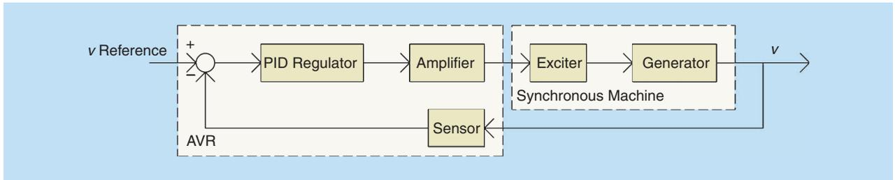
Figure 4. The voltage control cycle block scheme.
