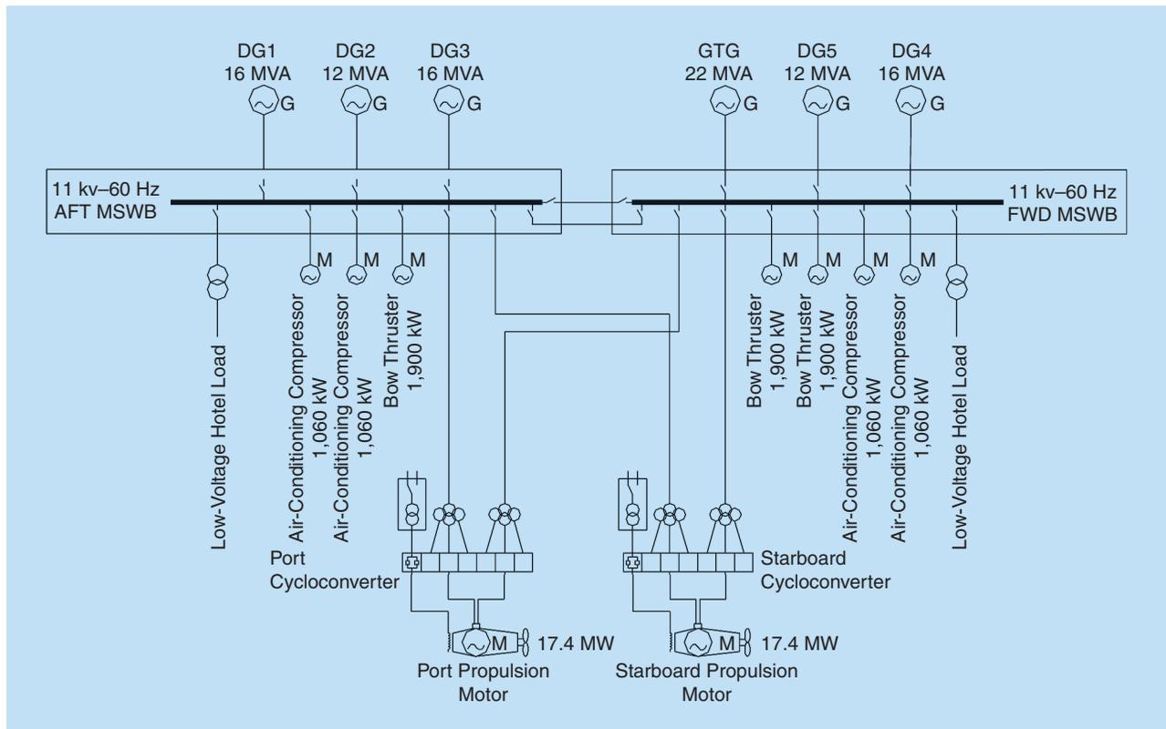
Figure 1. The typical IPS layout of an AES.
