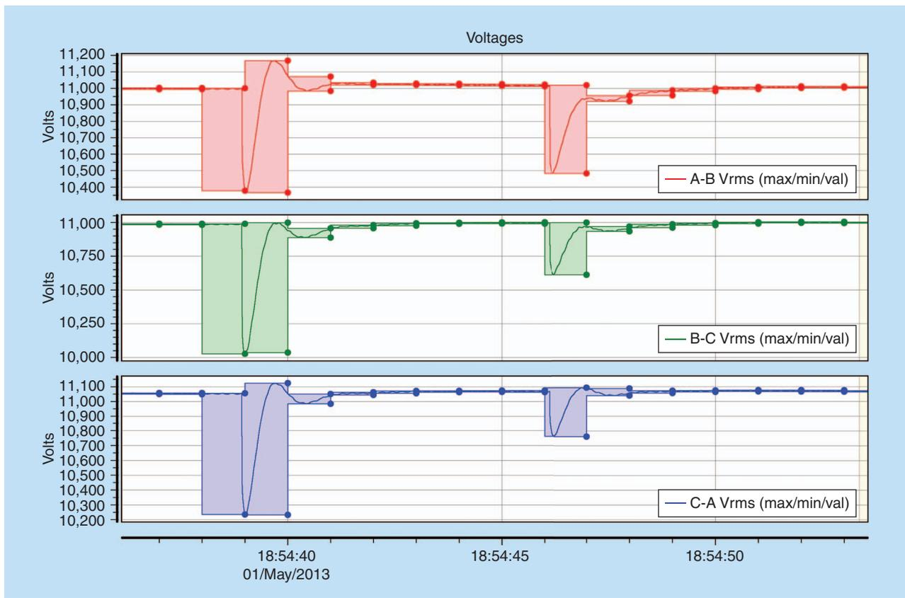
**Figure 12.** The main busbar voltage transients due to the propulsion transformer's inrush current.
