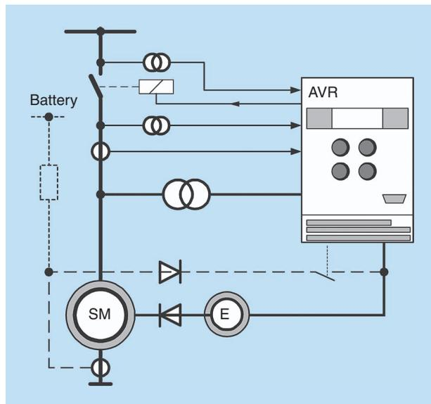
Figure 3. The AVR connection to the generator set (SM: generator; E: exciter).
