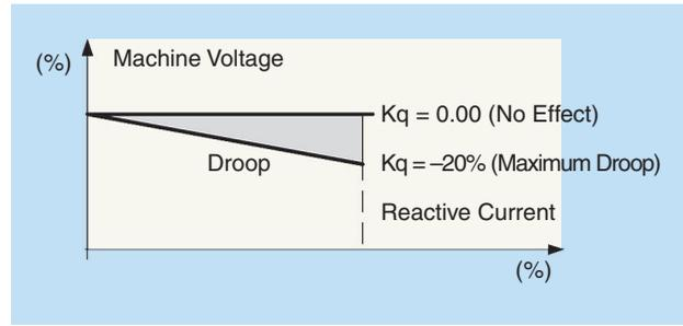
Figure 6. The reactive power-based voltage droop.
