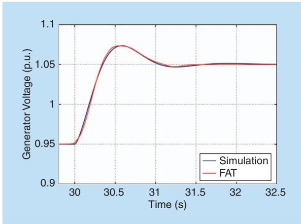
**Figure 16.** A diesel generator factory acceptance test (FAT) and simulation confrontation, no-load voltage reference step variation.
