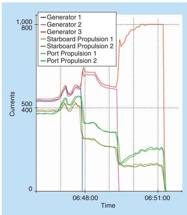
**Figure 15.** The experimental record of generator (1,000-A scale) and propulsion (800-A scale) currents during the incident leading to blackout.
