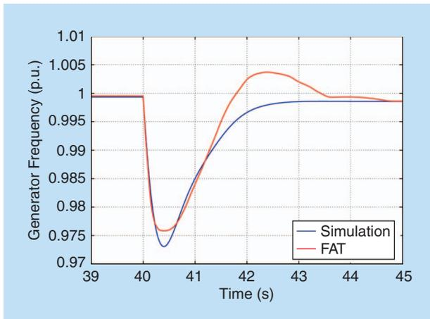
**Figure 17.** A diesel generator FAT and simulation confrontation, active load step variation.
