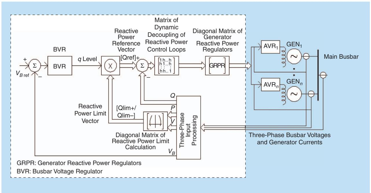
Figure 10. The possible architecture of an MIMO voltage and a reactive integrated regulator.
