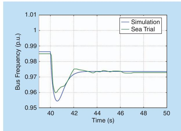
**Figure 19.** The sea trial and simulation confrontation of the generator's parallel operation, frequency transient due to one generator disconnection.
