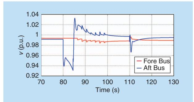
**Figure 23.** The simulated generator's busbar voltage transients during an emergency reconfiguration procedure.
