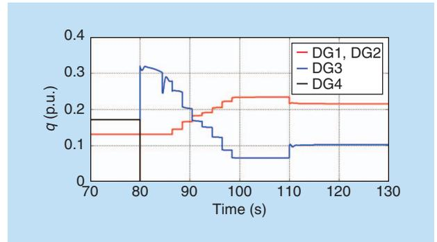
**Figure 22.** The simulated generator's reactive power transients during an emergency reconfiguration procedure.
