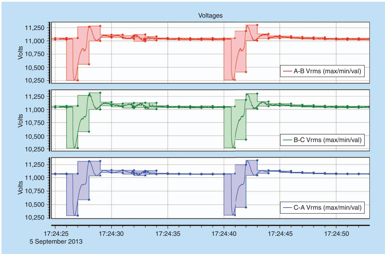
**Figure 11.** The main busbar voltage transients due to two 2.2-MW thrusters started up on an IPS with 88 MW total generator power.
