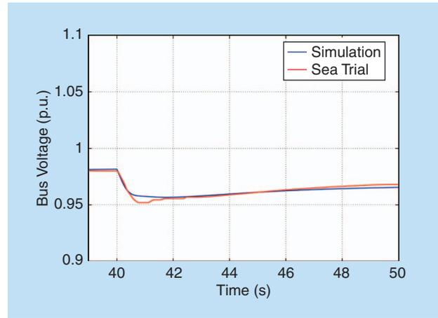
**Figure 18.** A sea trial and simulation confrontation of the generator's parallel operation, voltage transient due to one generator disconnection.
