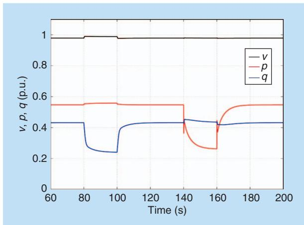
**Figure 9.** The diesel generator responses due to inverter-based generator references step variations.
