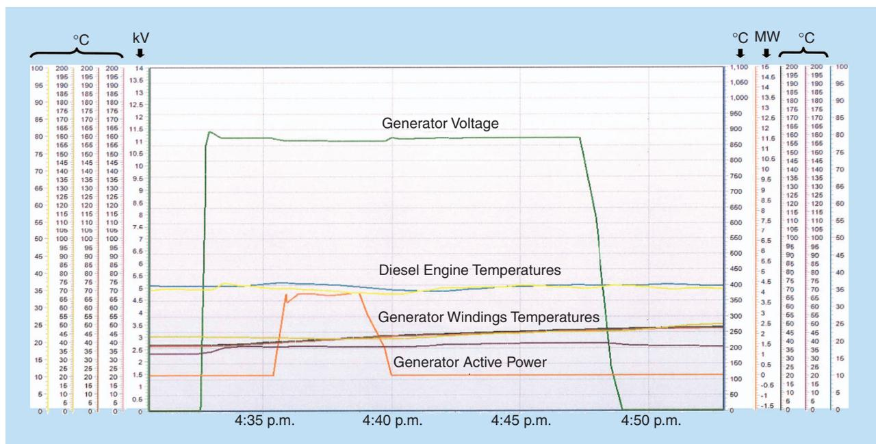
Figure 2. The ship's automation print screen of a generator's main variables during a maneuvering phase.
