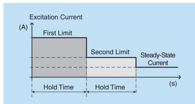
**Figure 14.** The AVR's time-based excitation current-limiting thresholds.
