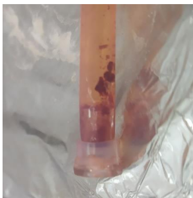
Figure 81 Microgels precipitation inside Float-A-Lyzer™ device after 52h of release. The purple colour is related to the presence of DOX inside the polymer precipitate.
