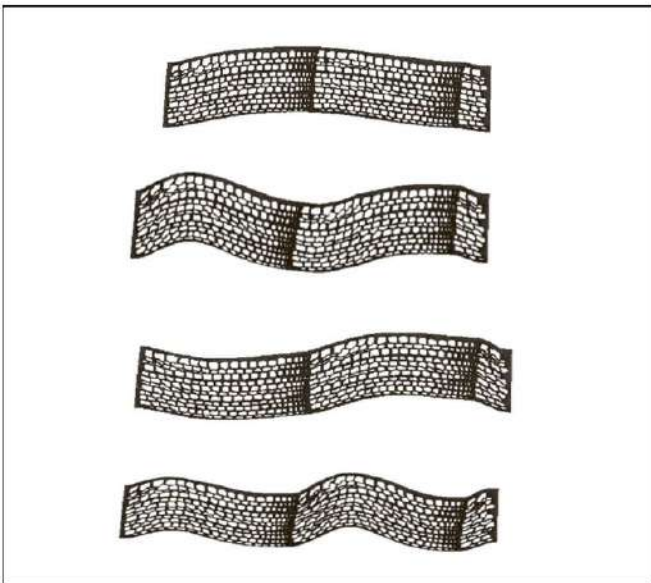
Figure 11. Graphical representation of the first four modes, referred to microstructure 2.
