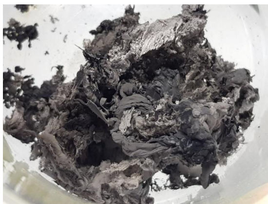
Fig. 1. Macroscopic appearance of MIM obtained by decomposition of \text{Fe}(\text{CO})_5
