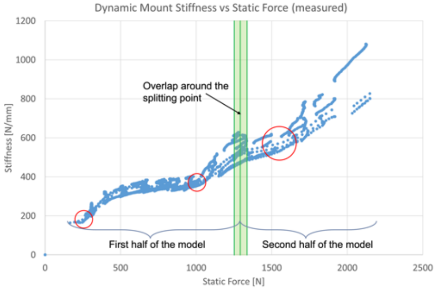
Figure 26: Multiple inflection points in a typical static force - dynamic stiffness diagram. The inflection points are highlighted with red markers. The domain is divided into two halves, identifying a static preload value as the splitting point. In the vicinity of such a point the two generated models are overlapped admitting a 2% superposition.
