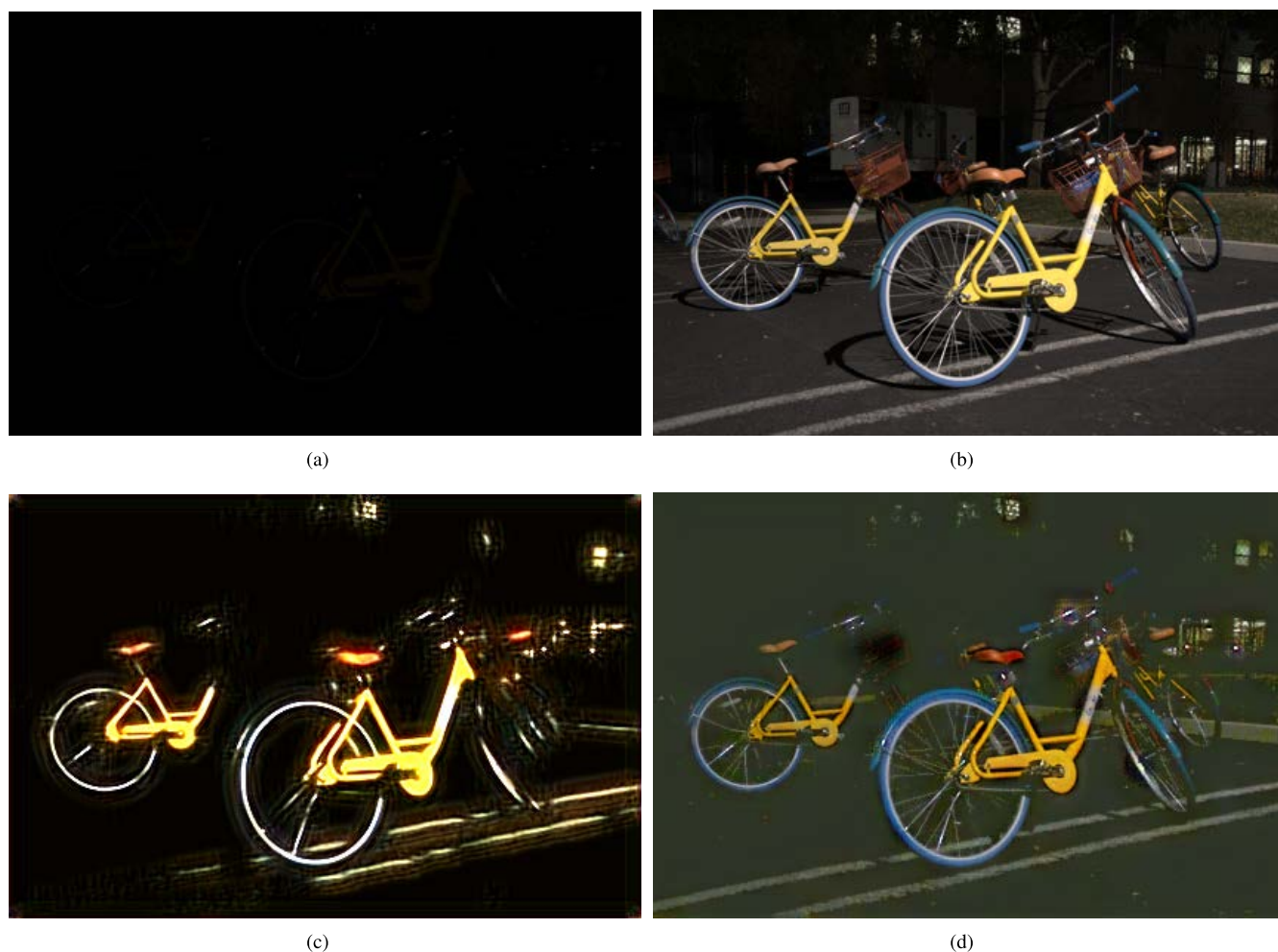
FIGURE 20. (a) Original low light RAW; (b) ground truth; and RAW image processed with (c) MBLLEN and (d) D2BGAN.
