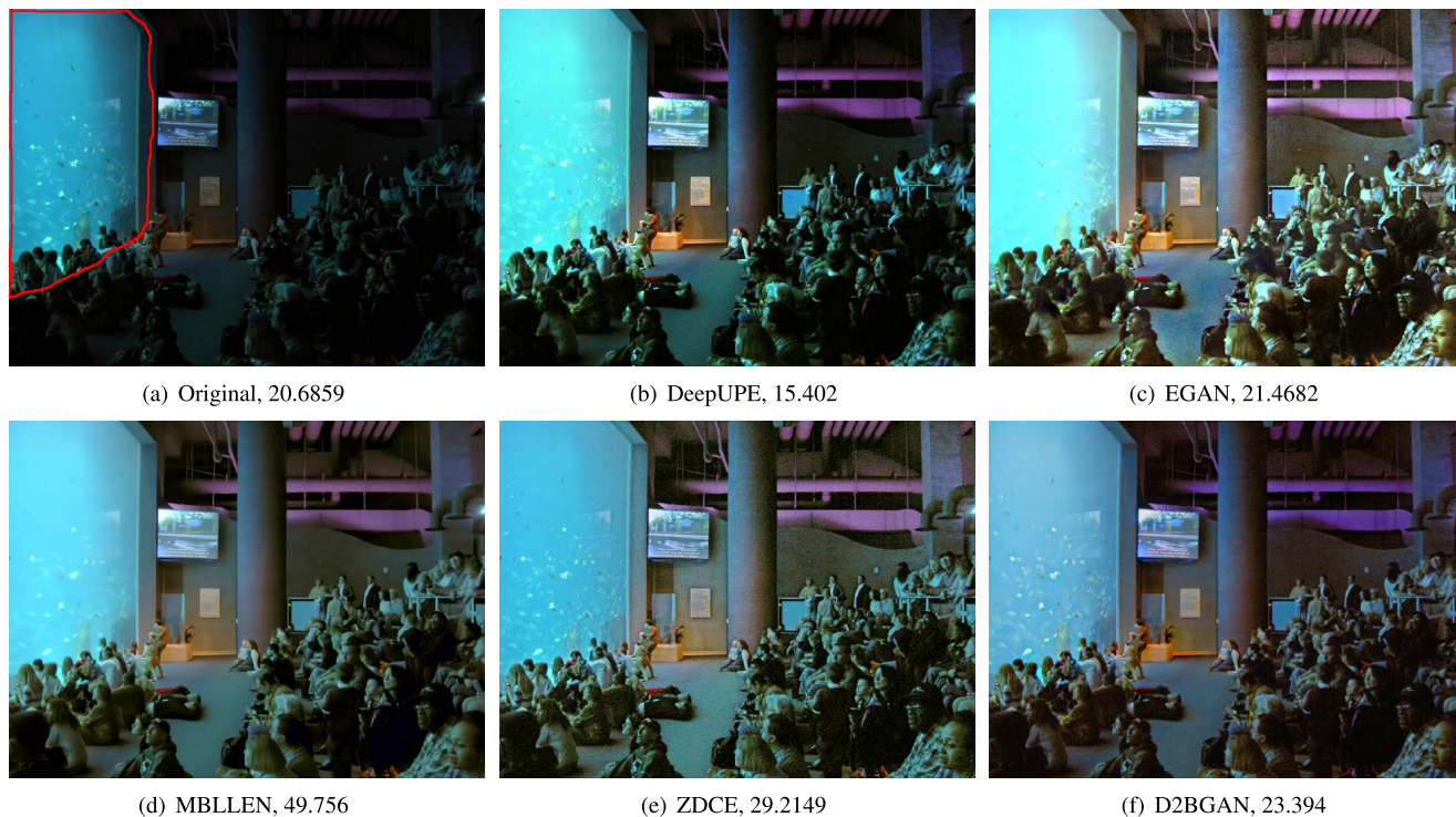
FIGURE 13. A strong contrast in the aquarium region (shown with red border in the original image) is observed in the DeepUPE and EGAN images. The considerably poor contrast results in a poor PIQE score for D2BGAN.
