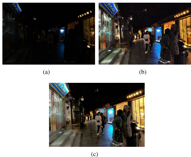
FIGURE 1. (a) Original dark image, (b) processed image with LIME (noise amplified), and (c) processed image with MBLLEN (artifacts due to smoothing).
