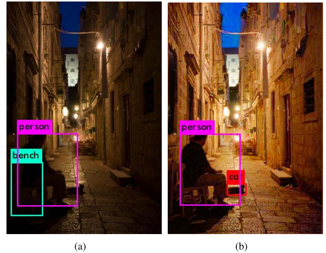
FIGURE 18. Face and object detection performances on original and pre-processed image from ExDark dataset. (a) is original while (b) is the processed version using D2BGAN.
