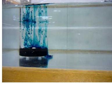
Figure 1.7: Side view of a Taylor columns experiment
