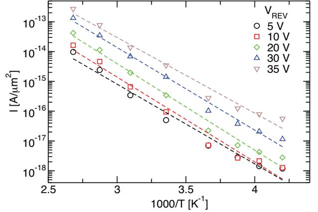
Fig. 5. Arrhenius plots of the dark current for several  $V_{REV}$  values. Curves show linear behavior down to low temperatures where they start to deviate likely because a temperature independent component enters into play.
