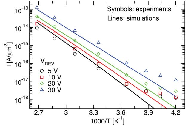
Fig. 8. Arrhenius plots simulated with  $\tau_n = \tau_p$  as in Eq. 5 and with  $E_T = E_i$ . Simulations now reproduce the experiments for different  $V_{REV}$ . A power-law temperature dependence is assumed to model the lifetimes (Eq. 5,  $\tau_{300K} = 0.39$  ns,  $\alpha = 6.06$ ). At low  $T$ , the experiments deviate from the linear behavior most likely because of the arise of a temperature independent component not included in simulations.
