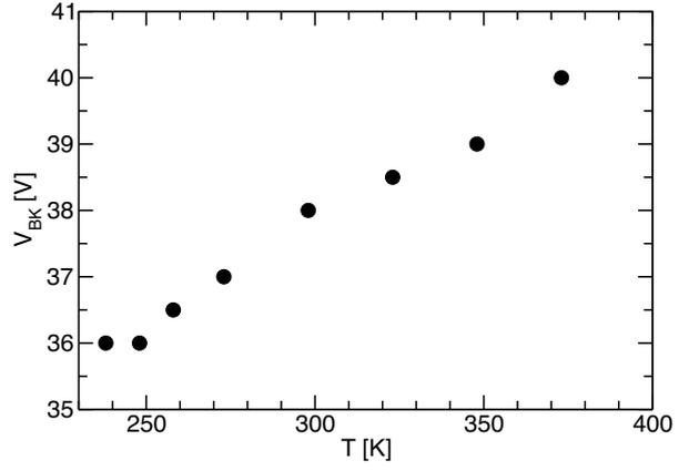
Fig. 4. Breakdown voltage versus  $T$  curve: the positive temperature coefficient confirms the avalanche multiplication process.
