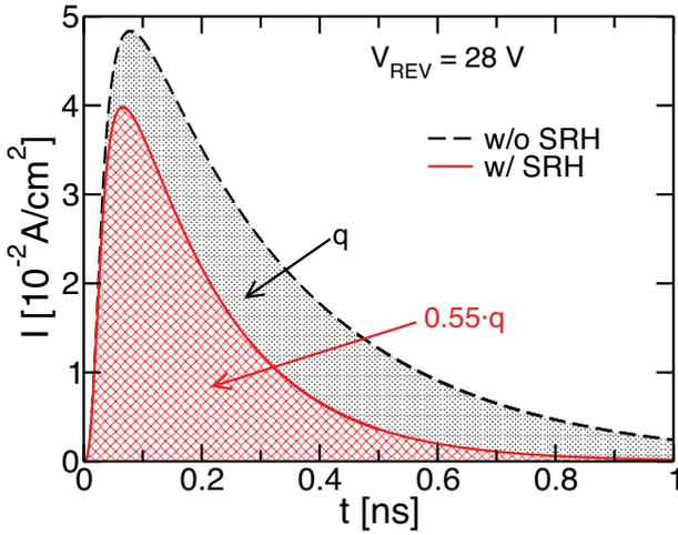
Fig. 13. Simulated current collected at the  $n$ -type contact as a function of time after the generation of an electron-hole pair in the middle of the absorption layer. The current is simulated including (red) or not (black) the SRH generation/recombination. At  $V_{REV} = 28$  V, the SRH process causes the loss of 45% of the photo-generated charge.
