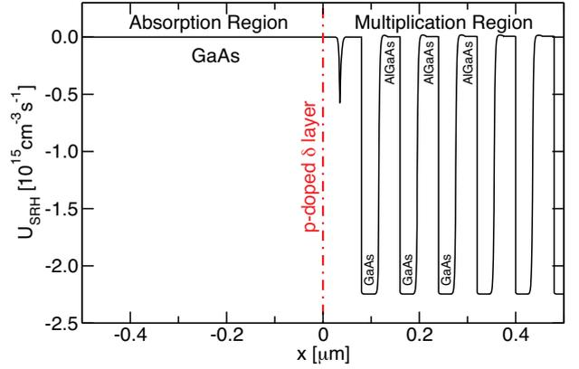
Fig. 9. SRH generation/recombination function along the device depth.  $x = 0$  corresponds to the  $p$ -doped  $\delta$  layer position that separates the absorption and multiplication regions. Note that carrier generation occurs in the GaAs layers of the multiplication region.  $V_{REV} = 20$  V.
