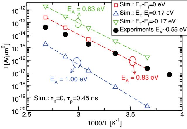
Fig. 7. Arrhenius plots simulated for  $V_{REV} = 20$  V assuming fixed  $\tau_n$  and  $\tau_p$  and variable trap energy depth  $E_T$ . For constant  $\tau_n$  and  $\tau_p$ , simulations cannot reproduce the measurements. Simulated  $E_A$  is always larger than in experiments.  $E_i$  is the Fermi level in the intrinsic semiconductor.
