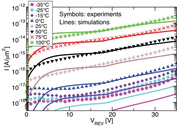
Fig. 10. Simulated IV curves with  $\tau_n = \tau_p$  as in Eq. 5. Simulations well reproduce the experiments, except at low  $T$ , when a temperature independent component most likely arises in the measurements.
