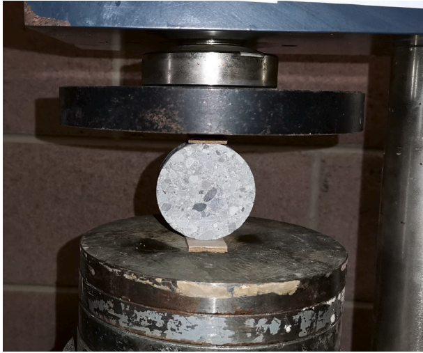
Fig. 9. Indirect tensile test on concrete disc.
