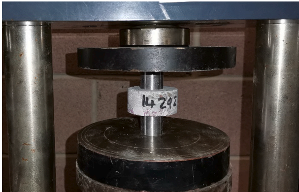
Fig. 7. Punching test setup on concrete disc.
