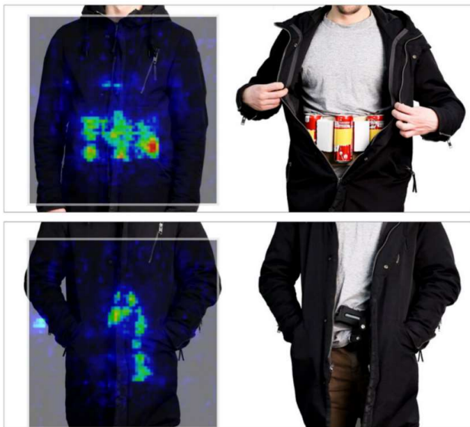
Figure 5 Imaging results of a real-life THz application for the detection of body-borne concealed threats, a belt with explosives and a gun [63].
