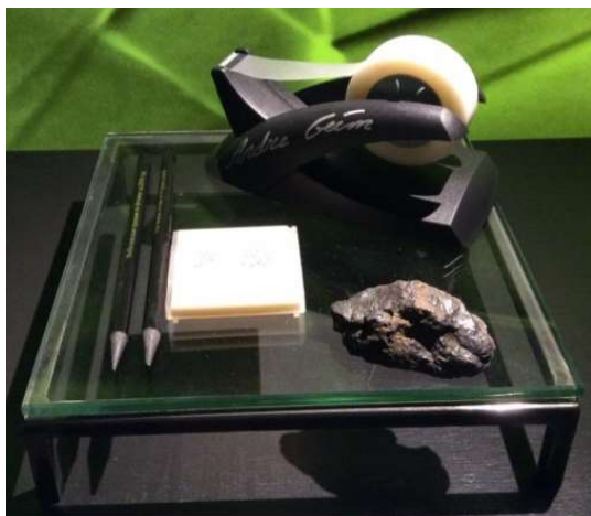
Figure 4 Display of the graphite, Scotch tape, and graphene transistor donated by the physicists to the Nobel Museum in Stockholm. [147]
