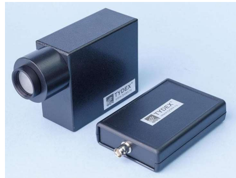
Figure 15 Left, schematic representation of a Golay cell and its components and (right) a commercial device [99] [100]. When the radiation hit the absorber, the gas sealed in the chamber is heated and expands correspondingly. The expansion of the elastic membrane is then measured through an optical system
