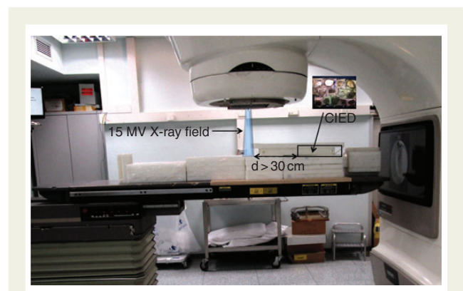
Figure 2 One of the two anthropomorphic phantoms (Ryan) designed for neutron dosimetry according to the indications of the International Commission on Radiological Protection, 8 the minimum distance between cardiac implantable electronic devices (CIED), positioned under a polyethylene layer of 3 cm (simulating for neutrons the adipose tissue and skin) and the radiation field (30 cm) is pointed out.
