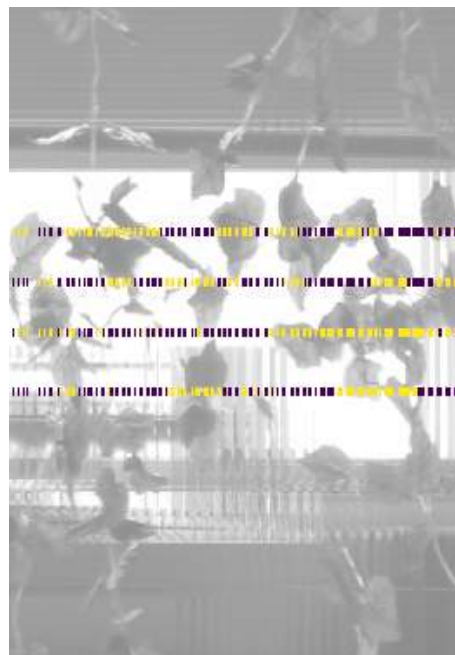
Figure 4. Collected data superimposed on a detail of the panoramic image of the synthetic vineyard: yellow points correspond to reflected IR rays, violet points to non-returning rays.
