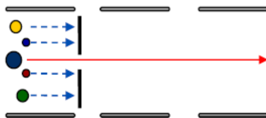
Figure 19. Schematic representation of the triple quadrupole analyzer in Q1MI configuration.
