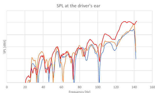
Figure 12: SPL perceived at the driver's ear — Measured SPL with isolated hoses — Synthesized SPL isolating the hoses — Measured SPL including the hoses contribution
