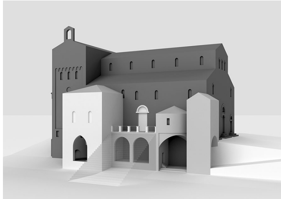
Fig. 2 Volumetric 3d reconstruction of the historical phases: in dark grey the romanesque church, in light grey the chapels built during the XIII century with the hypothetical staircase semitransparent
