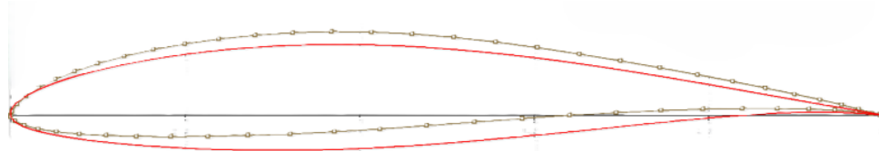
Figure 3. Eppler 393 (red) and NACA 63412 (brown) geometries (XFLR5).
