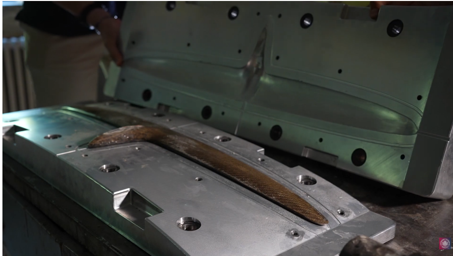
Figure 23. Taking the rudderfoil out of the mould (University of Trieste, 2023).
