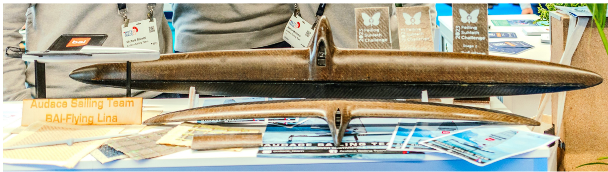
Figure 24. First couple of Audace flax fiber foils (METSTRADE 2023).
