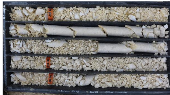
Figure 3. Core drill in the white limestones “Marmorino” in the “Valmadonna-Pedemonte” quarry.
