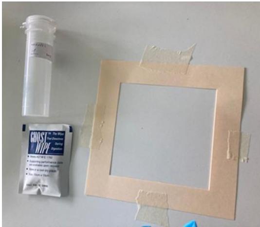
Figure 4: wipe samples 10x10 cm frame, ghost wipe and sample vial
