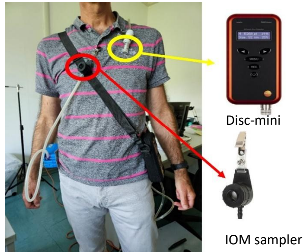
Figure 2: sampler placement on the worker
