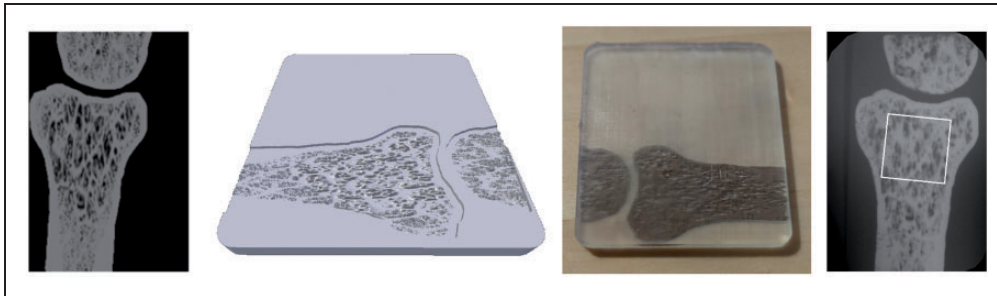
Figure 3. Type-B chips. (a) Starting image; (b) CAD drawing; (c) 3D printed chip; (d) radiogram.
