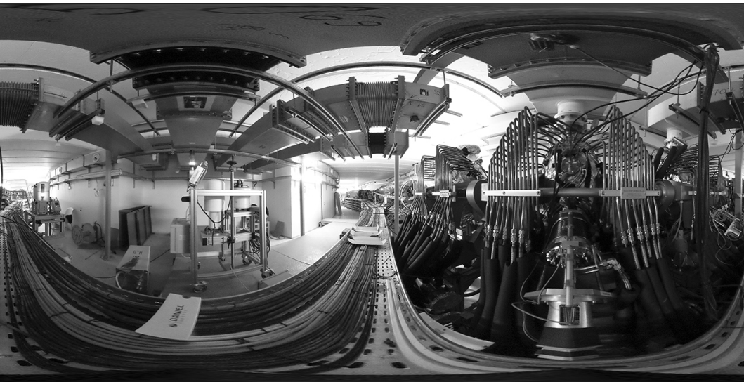
Fig. 3. Overview of the inside of the tunnel of the SESAME storage ring. The devices on the right are three of the four cavities made in Italy with part of Italy's financial contribution to SESAME.
