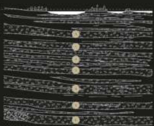
B. Stratigraphy of the Venetian subsoil The diagram above illustrates the stratigraphy of the Venetian subsoil. From a geological point of view, the subsoil of the lagoon is a multi-lake system characterized by an alternation of clay-silt impermeable layers and sandy layers. In the first 350 metres of depth, the latter house the Venetian aquifer that was affected by the artesian exploitation carried out for the construction of the first industrial nucleus of Porto Marghera starting in the Thirties of the 20th century. After the war, exploitation also affected the sixth aquifer, leading not only to a lowering of the piezometric level but also to the lowering of the soil with an average value of 8 millimetres per year.
