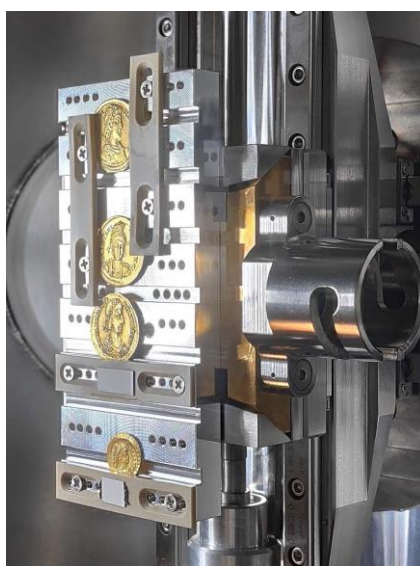
Figure 6: The four gold coins analysed in this work, inside the UHV chamber at the XRF beamline at Elettra Synchrotron.
