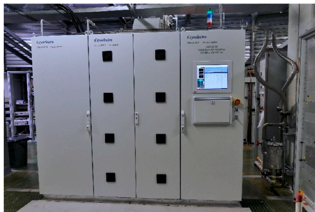
Fig. 38. 130 kW 500 MHz solid state amplifier.
