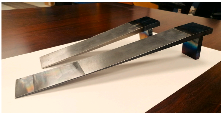
Fig. 6. ABH Model 1 and Model 2 prototypes manufactured for the experiment.
