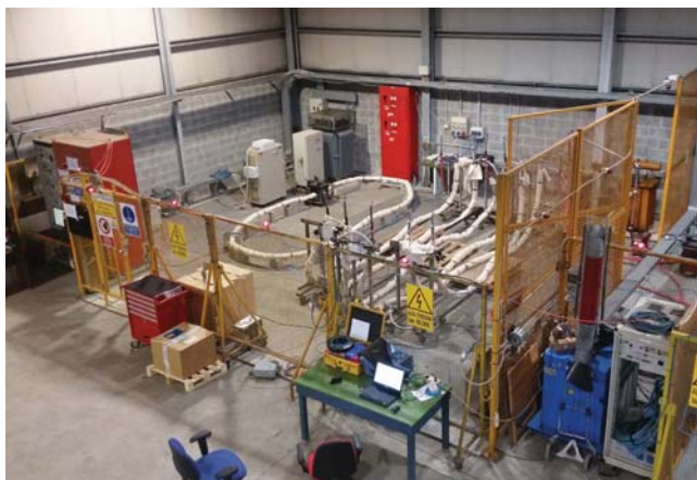
Figure 2 - Experimental set-up: view of the mirror ring and the part of the main ring with the six new joints (the other six from service are on the right part of the circuit and not visible in the picture).
