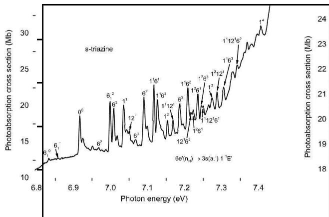
Fig. 4. Photoabsorption cross section of s-triazine, encompassing the excitation range 6.80–7.45 eV, showing structure due to the  $6e^0(n_n) \rightarrow 3s(a_1^0) 1^1 E^0$  transition. Experimental excitation energies and assignments are given in Table 5.
