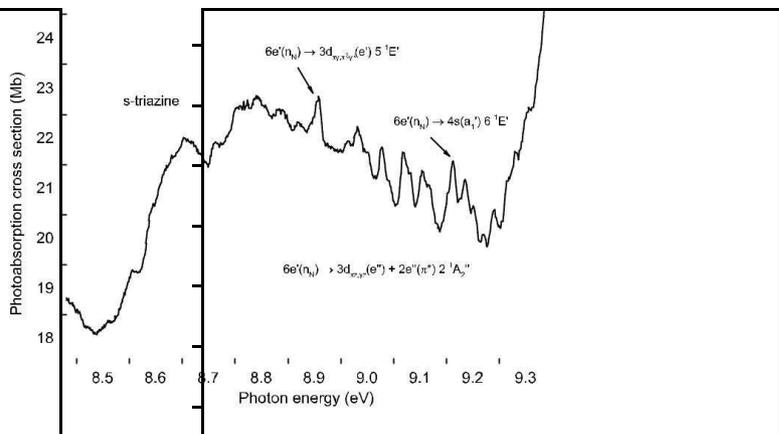
Fig. 5. Photoabsorption cross section of s-triazine, encompassing the excitation range 8.5–9.3 eV, showing structure due to Rydberg states belonging to series converging onto the  $X \tilde{E}$  state threshold.
