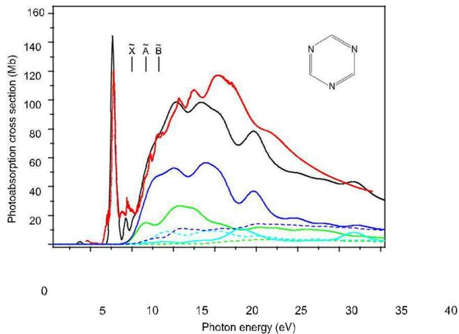
Fig. 1. The experimental (red) and convoluted TDDFT (black) photoabsorption cross section of s-triazine. The calculated partial final continuum contributions ( $-a_1^0$  (green),  $-a_2^0$  (cyan),  $-e^0$  (blue),  $-a_1^{00}$  (green),  $-a_2^{00}$  (cyan),  $-e^{00}$  (blue)) are shown.
