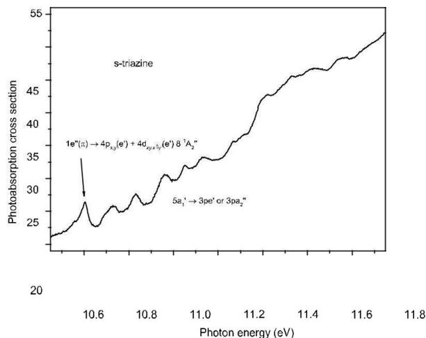
Fig. 7. Photoabsorption cross section of s-triazine encompassing the excitation range 10.5–12.0 eV. The structure above 11 eV may involve excitation from the  $5a_1^0$  orbital.
