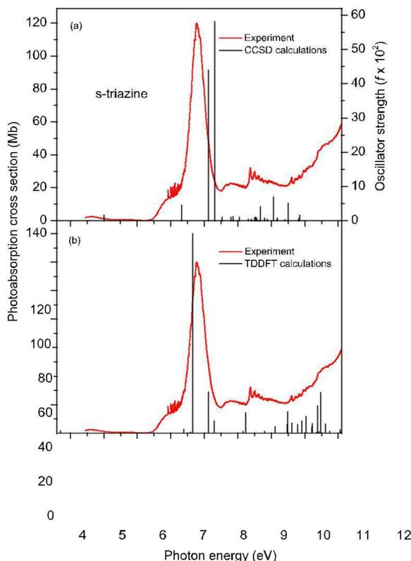
Fig. 2. (a) The experimental photoabsorption cross section of s-triazine (red) and the CCSD predicted oscillator strengths (black), plotted as vertical bars, using the results given in Table 4. (b) The experimental photoabsorption cross section of s-triazine (red) and the TDDFT predictions (black), plotted as vertical bars, using the results given in Table 2. (For interpretation of the references to colour in this figure legend, the reader is referred to the web version of this article.)
