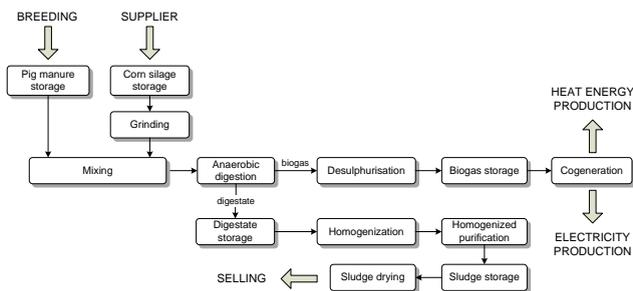
**Fig. 1 – Block diagram of a traditional anaerobic digestion plant**
