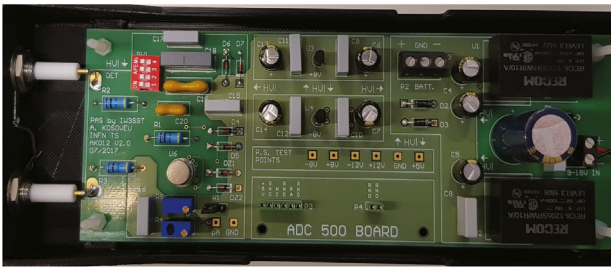
Fig. 10. Picture of the ammeter board with components installed ready for the preliminary functional tests.
